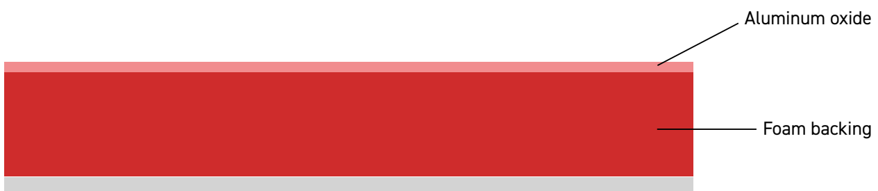
2D drawing of the grain structure of the DRYFINISH Multihole Foam Abrasive Discs.
