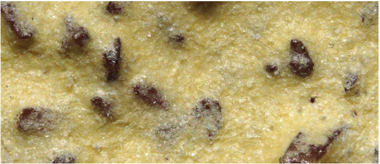
Microscopic view of the grain pattern of the MULTIPURPOSE Paper Abrasive Discs.
